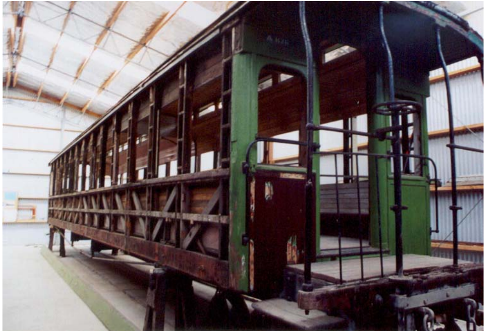
Car # 48 undergoing restoration at Silver Stream
