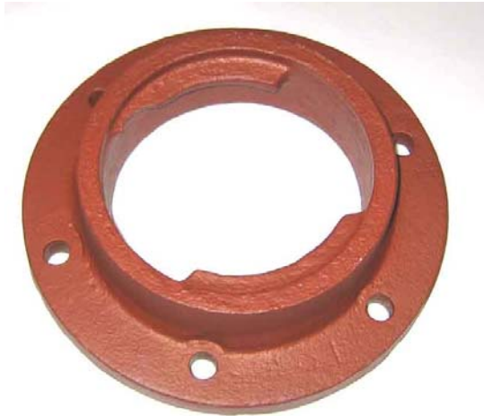
The smoke box inspection hatch we recovered.
